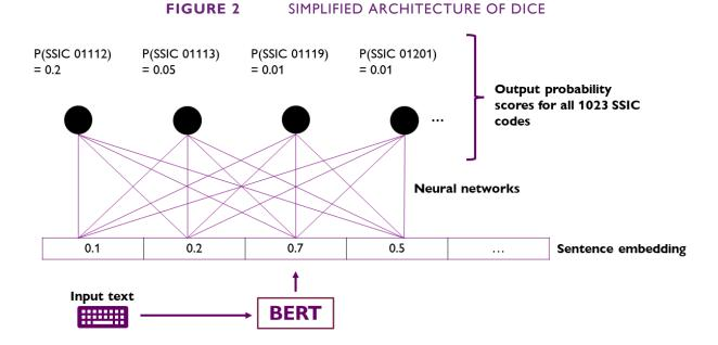
text including 2.5 billion words from the English Wikipedia. BERT models utilise sentence embeddings to support various downstream tasks such as predicting SSIC codes, by adding a neural network layer on top of them (Figure 2). The entire network is then fine-tuned by training on the task-specific data (i.e., descriptions of firm activities and corresponding SSIC codes).
